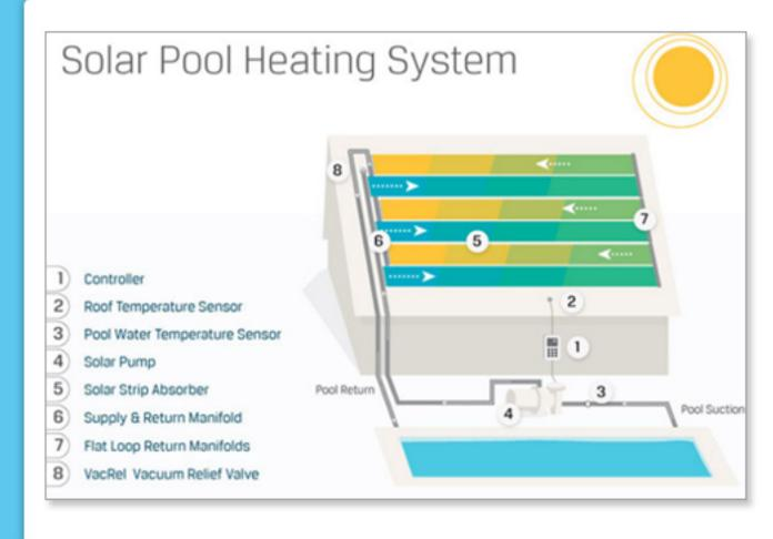
The MS3D solar controller is a set and forget user friendly digital differential temperature controller designed to give trouble free pool heating from the sun. Once the comfort temperature is set, the MS3D id left to itself to calculate energy efficient solar pool heating. The MS3D features include delayed start up to allow the filter pump to fully prime, tropical and winter modes and the availability tofully over ride the controller, ensuring many years of efficient pool heating.
